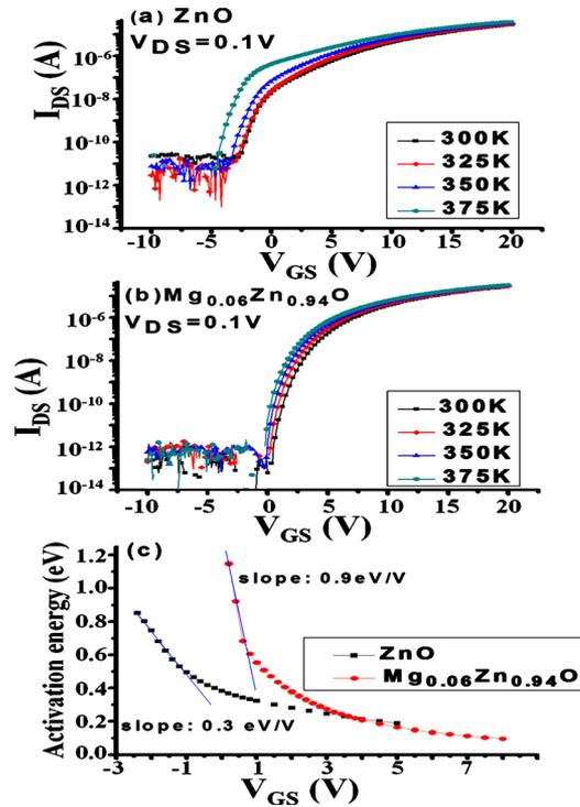
FIG. 3. (Color online) The evolution of transfer characteristics of (a) ZnO TFT and (b)  $\text{Mg}_{0.06}\text{Zn}_{0.94}\text{O}$  TFT at different temperatures, ranging from 300 to 375 K. (c) The extracted activation energies as a function of  $V_{\text{GS}}$  for ZnO and  $\text{Mg}_{0.06}\text{Zn}_{0.94}\text{O}$  TFTs.
