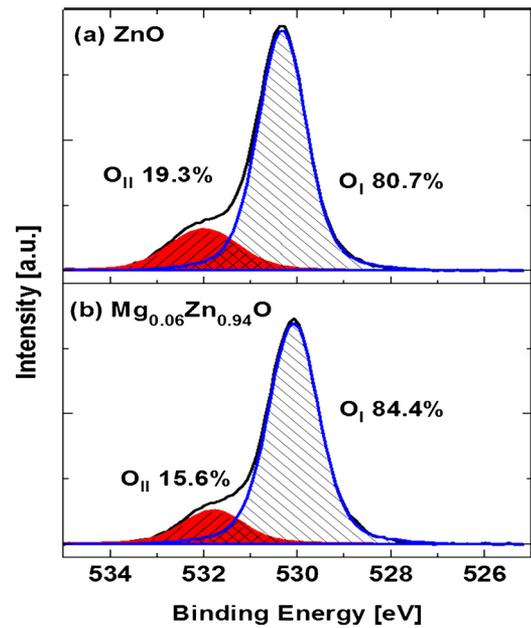
FIG. 2. (Color online) The  $O_{1s}$  peaks in the XPS spectra of (a) pure ZnO and (b)  $Mg_{0.06}Zn_{0.94}O$  channel layers. The original  $O_{1s}$  peaks were deconvoluted by Gaussian fitting into two subpeaks including  $O_I$  (oxygen bonded with Zn) and  $O_{II}$  (oxygen vacancy related). The peak area of  $O_{II}/(O_I+O_{II})$  is reduced after incorporation of 6% Mg into the ZnO.
