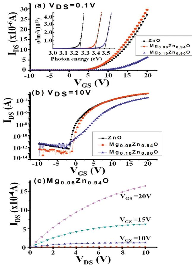
FIG. 1. (Color online)  $I_{DS}$ - $V_{GS}$  transfer characteristics of ZnO,  $Mg_{0.06}Zn_{0.94}O$ , and  $Mg_{0.1}Zn_{0.9}O$  TFTs: (a) in the linear region; the inset shows the  $\alpha^2$  vs  $h\nu$  curves of ZnO,  $Mg_{0.06}Zn_{0.94}O$  and  $Mg_{0.1}Zn_{0.9}O$ ; (b) in the saturation region; and (c) the  $I_{DS}$ - $V_{DS}$  characteristics of  $Mg_{0.06}Zn_{0.94}O$  TFTs.
