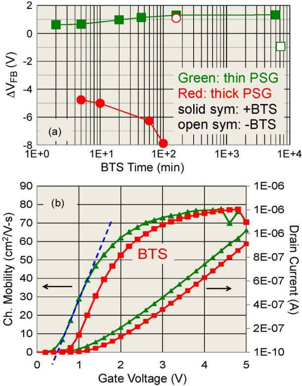
Fig. 3. (a) BTS-induced flatband voltage shifts ( $\Delta V_{FB}$ ) for PSG MOS capacitors. (b) Effects of positive BTS on thin PSG MOSFET threshold voltage and channel mobility. *BTS conditions*: 150 °C,  $+V_g$  ( $E_{ox} = 1.5 \text{ MV/cm}$ ), and  $-1.5V_g$  for n-MOS capacitors; 150 °C, 8 h, and  $+V_g$  used for thin PSG MOSFETs.
