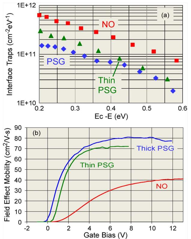
Fig. 2. (a) Interface trap densities for 4H-SiC MOS capacitors. (b) Channel mobilities for passivated 4H-SiC MOSFETs.
