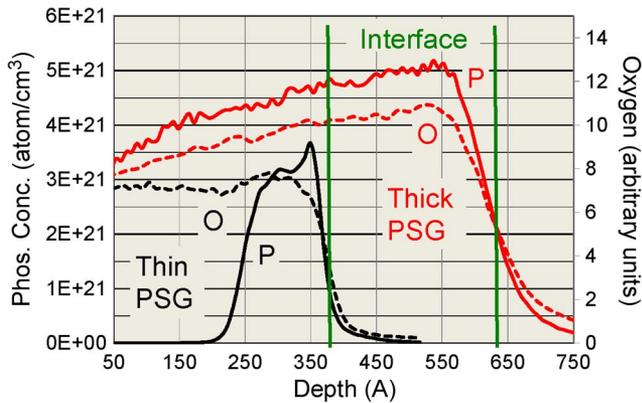
Fig. 1. SIMS profiles for PSG MOSFETs. The phosphorous concentrations are accurate only in the oxide and PSG layers.
