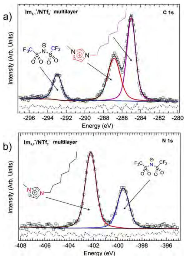
FIG. 4. C 1s and N 1s core levels measured on a thick film of Im<sub>8,1</sub><sup>+</sup>/NTf<sub>2</sub><sup>−</sup> deposited in UHV on gold. The deconvolution of the core levels and their attribution is indicated. The dotted line indicates the fit residue.
