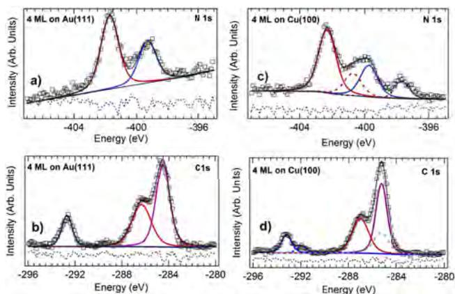
FIG. 7. N 1s and C 1s core level spectra for 4 ML thickness on the Au(111) ((a) and (b), respectively) and Cu(100) ((c) and (d), respectively) surfaces (open squares). Color coded spectral assignments are given in Fig. 4.
