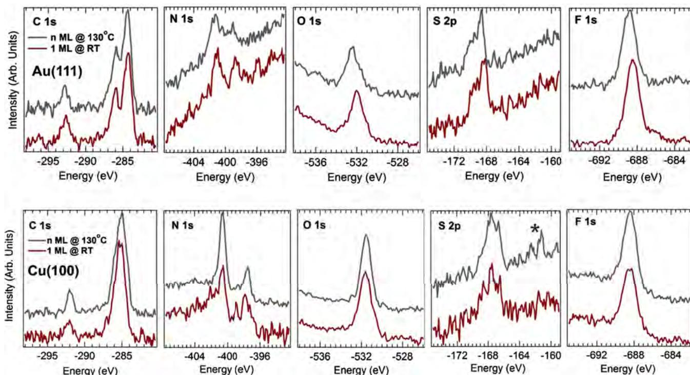
FIG. 9. Comparison of the C 1s, N 1s, O 1s, S 2p, and F 1s XPS core levels, measured for a 1 ML coverage deposited at room temperature and on a multilayer annealed to 130 °C for 10 min on Au(111) (top) and Cu(100) (bottom).
