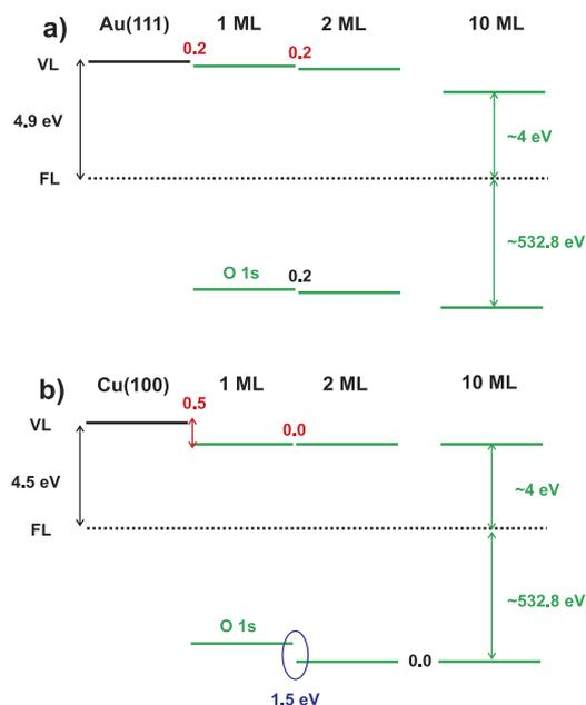
FIG. 8. Schematic energy diagram representing the vacuum level (VL), the Fermi level, and a typical core level, O 1s, positions as a function of the IL layer thickness on the (a) Au(111) and (b) Cu(100) surfaces. Work function changes are indicated in red.
