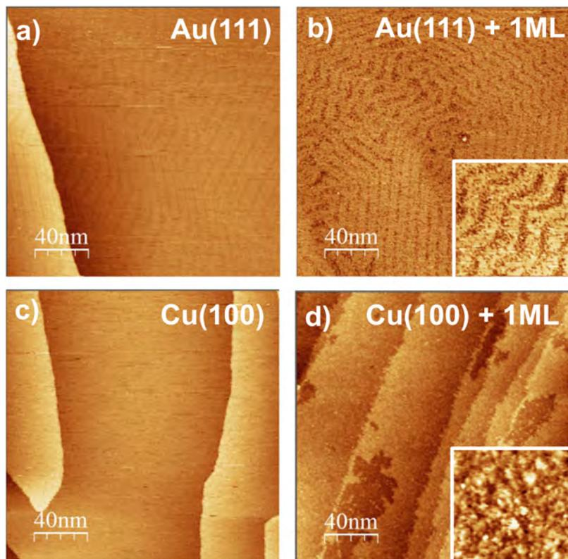
FIG. 2. STM images obtained on the Au(111) and Cu(100) surfaces, before ((a) and (c), respectively) and after deposition of a monolayer of the  $\text{Im}_{8,1}^+/\text{NTf}_2^-$  IL ((b) and (d), respectively). Insets show a  $40 \times 40 \text{ nm}^2$  area of the corresponding surfaces.
