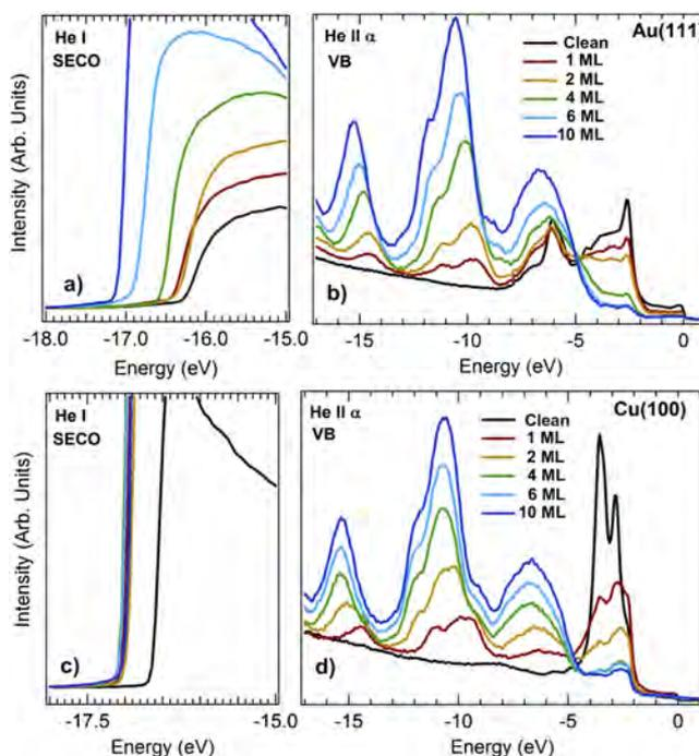
FIG. 5. UPS spectra of SECO and VB measured on the Au(111) ((a) and (b), respectively) and Cu(100) ((c) and (d), respectively) surfaces before and after sequential IL deposition.
