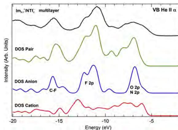
FIG. 3. VB spectra measured on a thick film of  $\text{Im}_{8,1}^+/\text{NTf}_2^-$  deposited in UHV on gold. The DOSs calculated for the ion pair and for individual ions are also shown, shifted in energy so as to match experimental features.
