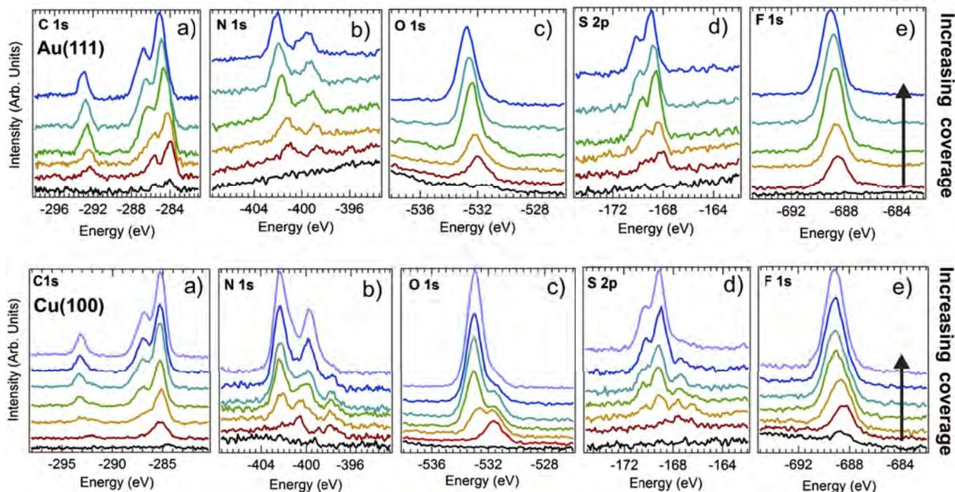
FIG. 6. XPS core levels for C 1s, N 1s, O 1s, S 2p, and F 1s, measured for clean surfaces and following subsequent deposition of the IL. Top: Au(111) surface; bottom: Cu(100) surface. Coverages are similar to the one of Fig. 5.
