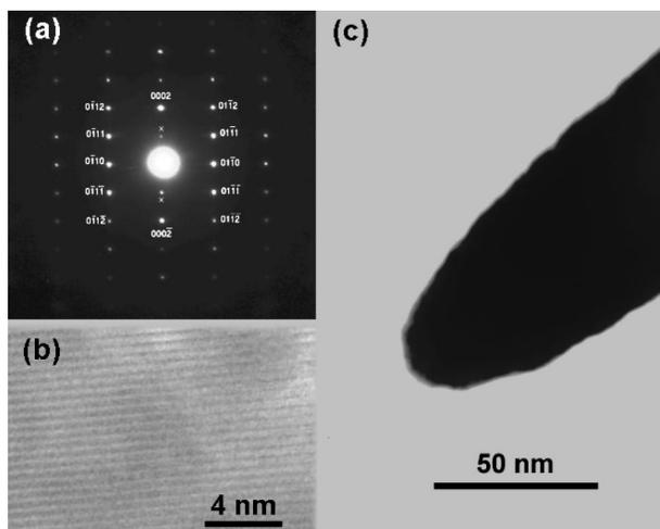
FIG. 2. (a) Selected area diffraction pattern of a single Ga-doped ZnO nanotip along the  $[2\bar{1}10]$  zone axis, (b) an image of a single-crystalline tip from high-resolution TEM, and (c) dark-field TEM image of a single Ga-doped ZnO nanotip.
