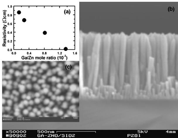
FIG. 1. (a) Measured resistivity of Ga-doped epitaxial ZnO films versus Ga/Zn mole ratios. (b) FESEM image of Ga-doped ZnO nanotips grown on fused silica substrate. (c) Top view of the ZnO nanotips.
