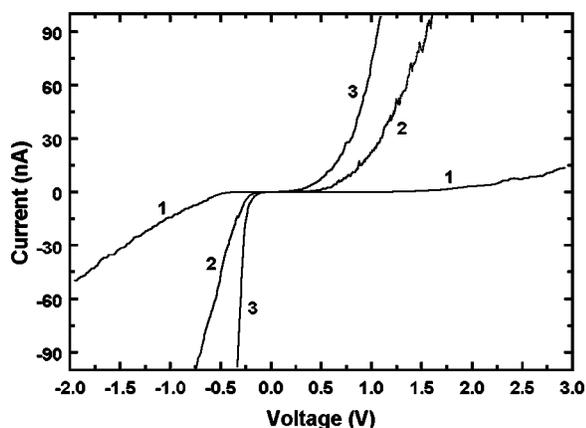
FIG. 4.  $I$ - $V$  spectra for the undoped and Ga-doped ZnO nanotips, where curves 1, 2, and 3 correspond to the spectra of undoped and Ga-doped ZnO nanotips with reference resistivities of 40  $\Omega$  cm (undoped), 0.58  $\Omega$  cm (Ga-doped),  $4.0 \times 10^{-3}$   $\Omega$  cm (Ga-doped), respectively.
