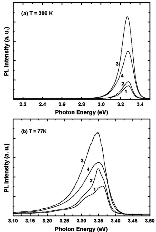
FIG. 3. (a) RT PL spectra of undoped and Ga-doped ZnO nanotips. (b) 77 K PL spectra of undoped and Ga-doped ZnO nanotips. Curves 1, 2, 3, and 4 correspond to the spectra of undoped and Ga-doped ZnO nanotips with reference resistivities of  $40\ \Omega\text{ cm}$  (undoped),  $0.58\ \Omega\text{ cm}$  (Ga-doped),  $4.0 \times 10^{-3}\ \Omega\text{ cm}$  (Ga-doped) and  $3.0 \times 10^{-3}\ \Omega\text{ cm}$  (Ga-doped), respectively.
