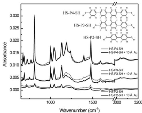
**Figure 1.** GI-FTIR spectra of HS-P4-SH, HS-P3-SH, and HS-P2-SH before (gray) and after (black) deposition of 10 Å Au. A vertical offset is introduced for clarity (0.003 and 0.010 units for HS-P3-SH and HS-P4-SH, respectively).
