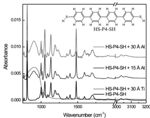
**Figure 2.** GI-FTIR spectra of pristine HS-P4-SH (black) and HS-P4-SH with 15 Å Al (dark gray), 30 Å Al (gray), and 30 Å Ti (light gray). A vertical offset for Al deposition is introduced for clarity.
