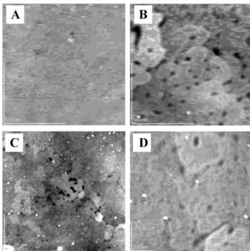
**Figure 3.** AFM images of HS-P4-SH before (panel A,  $1 \times 1 \mu\text{m}$ ) and after deposition of 30 Å Au (panel B,  $1 \times 1 \mu\text{m}$ ), Al (panel C,  $3.3 \times 3.3 \mu\text{m}$ ), and Ti (panel D,  $1 \times 1 \mu\text{m}$ ).
