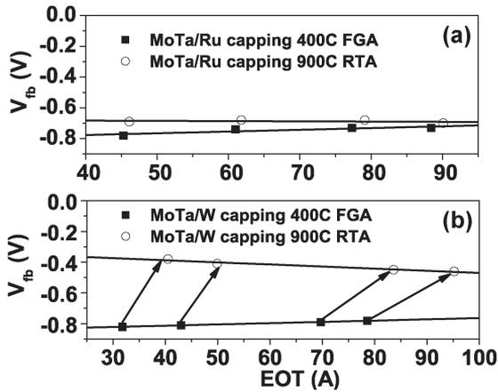
Fig. 1.  $V_{fb}$  versus EOT curves of (a) MoTa/Ru and (b) MoTa/W at 400 °C FGA and 900 °C RTA. The MoTa/Ru stack has stable work function values up to 900 °C, while the work function and EOT of MoTa/W increase after 900 °C RTA.
