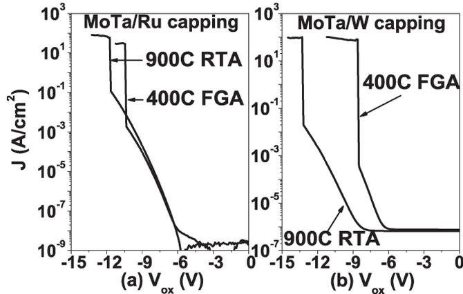
Fig. 2.  $I$ - $V$  curves of (a) MoTa/Ru and (b) MoTa/W at 400 °C FGA and 900 °C RTA, showing that MoTa/Ru has a similar  $I$ - $V$  at 400 °C FGA and 900 °C RTA, whereas the  $I$ - $V$  curve of MoTa/W shifts to lower values after 900 °C RTA.
