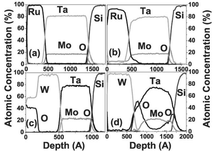
Fig. 3. AES depth profiling of (a) MoTa/Ru at 400 °C FGA, (b) MoTa/Ru at 900 °C RTA, (c) MoTa/W at 400 °C FGA, and (d) MoTa/W at 900 °C RTA. MoTa/Ru has a sharp interface with  $\text{SiO}_2$  at both 400 °C FGA and 900 °C RTA, indicating good thermal stability. MoTa gets oxygen from  $\text{WO}_x$  at 900 °C RTA.  $\text{WO}_x$  forms during the 400 °C FGA.
