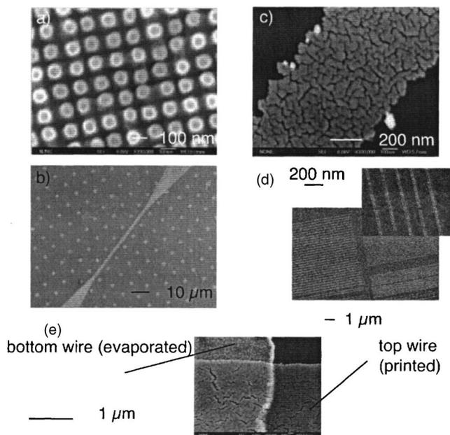
FIG. 6. Patterns generated by nTP: (a) gold dots of 100 nm diameter, (b) continuous gold line, (c) microscopic cracks seen at larger magnification do not break the electrical continuity of the wide lines, (d) narrow lines, which are disconnected due to cracks in the metal layer, and (e) cross junction of bottom evaporated gold line with a top printed electrode. The SAM on top of the bottom electrode serves both as electrical isolation and binding partner for the top electrode.
