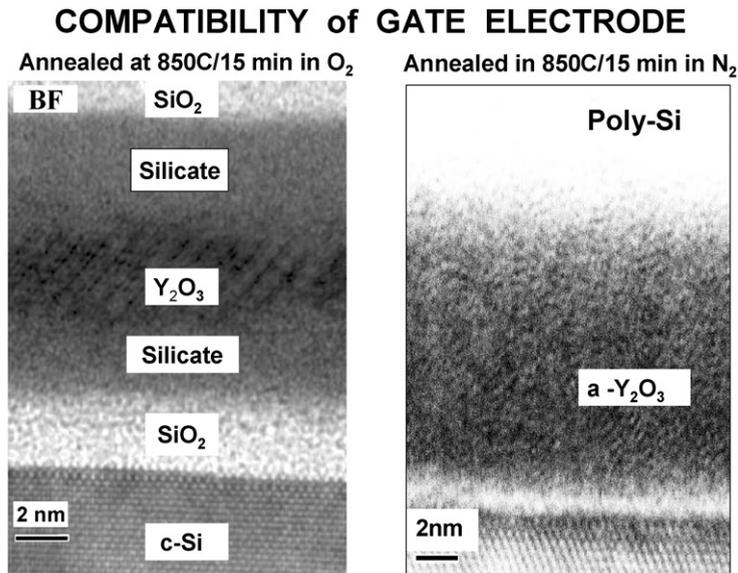
Fig. 6. BF-STEM cross sectional images for: (a) O<sub>2</sub> annealed, and (b) N<sub>2</sub> annealed a-Si/Y<sub>2</sub>O<sub>3</sub>/c-Si stacks at 850°C for 15 min.
