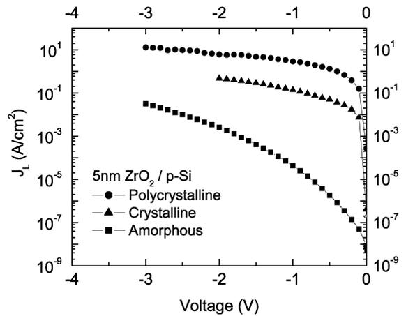
Fig. 2. Morphology dependence of leakage current density vs. voltage for 5.0 nm  $ZrO_2$  films of varying microstructure on (100) Si.
