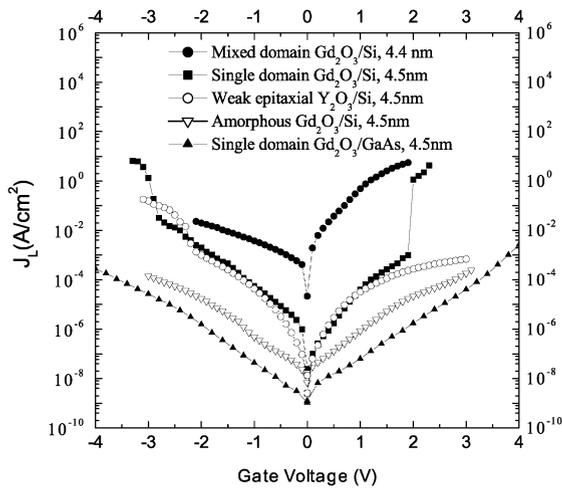
Fig. 1. Morphology dependence of leakage current density  $J_L$  vs. voltage for 4.5 nm  $Gd_2O_3$  and  $Y_2O_3$  films of varying microstructure on (100) Si and (100) GaAs.
