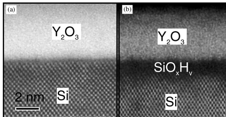
Fig. 4. (a) ADF-STEM image of an a-Si/ $Y_2O_3$ /c-Si stack, which is thick enough so that surface reaction layers are not visible. (b) The same a-Si/ $Y_2O_3$ /c-Si sample in a thinner region. Not only has a hydroxide formed on the entrance and exit surfaces, but the capping layer has also been milled away and the hydroxide reaction layers dominate the interface contrast.
