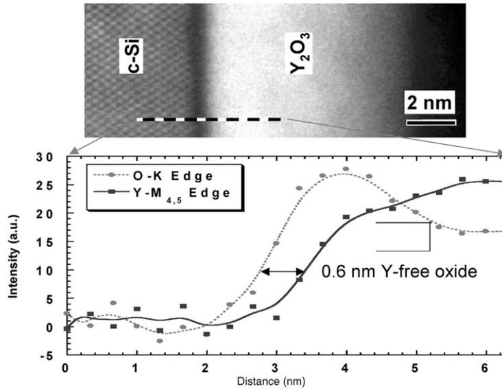
Fig. 5. Oxygen-K edge and yttrium-M<sub>4,5</sub> edge of EELS spectra for an a-Si/Y<sub>2</sub>O<sub>3</sub>/c-Si film, showing a SiH<sub>x</sub>O<sub>y</sub> hydroxide near the Si interface.
