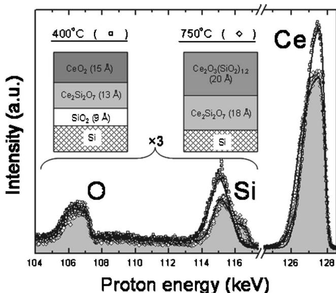
FIG. 3. MEIS energy spectra for ceria films annealed at 400 °C (squares) and 750 °C (diamonds). The solid lines show simulated spectra obtained using model structures sketched in the inset.
