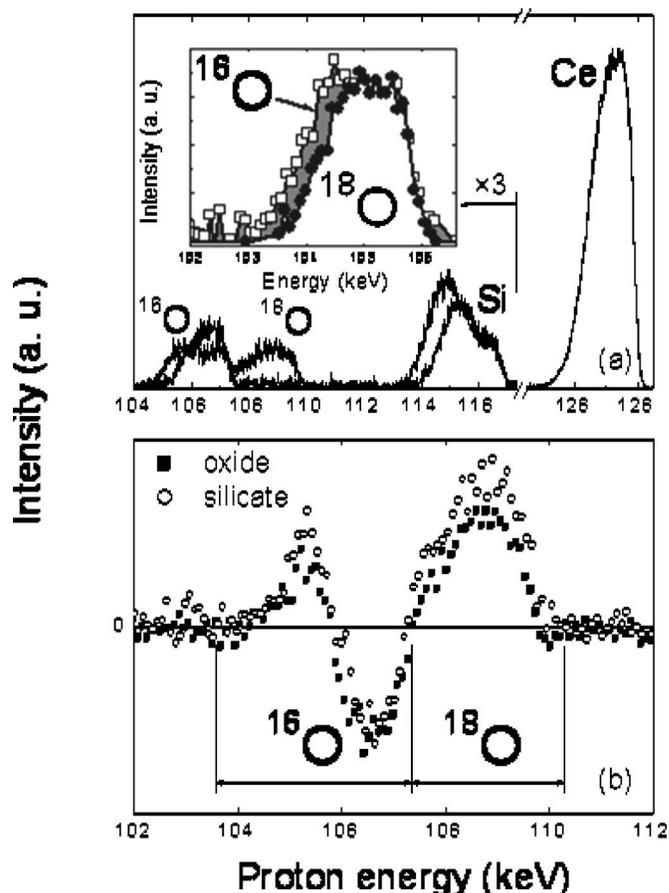
FIG. 4. The upper graph shows MEIS energy spectra from the cerium silicate film before and after reoxidation in <sup>18</sup>O<sub>2</sub>. The inset shows the <sup>18</sup>O peak superimposed on the <sup>16</sup>O peak in the same spectrum by shifting its energy position by the known difference in scattered energy. The scattering angle was 133°. The lower graph shows a difference spectra in the oxygen energy region for the films annealed at 400 °C (filled squares) and 750 °C (open circles).
