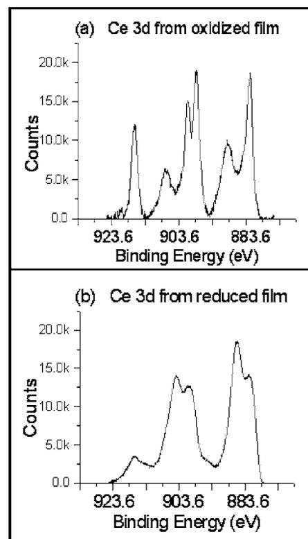
FIG. 1. Ce 3d XPS spectra (after linear background subtraction) from cerium oxide showing (a) mostly Ce<sup>4+</sup> character and (b) mostly Ce<sup>3+</sup> character.
