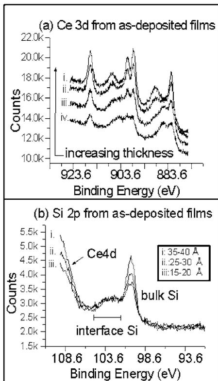
FIG. 2. XPS spectra from three films of varying thickness, deposited with similar oxygen exposure:  $6.6 \times 10^{-6}$  Torr  $O_2$  for 10 min. (a) Ce 3d spectra showing progressively decreasing  $Ce^{4+}$  character as the film gets thinner. (b) Si 2p spectra showing similar interface signals for the three sample thicknesses.
