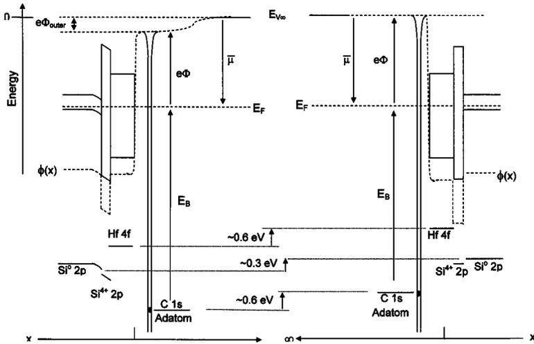
FIG. 9. The electrostatic potential distribution across gate stack (a) as-deposited (b) after a forming gas anneal at 400 °C.
