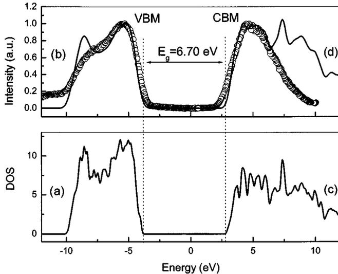
FIG. 4. (a) Theoretical valence band density of states (DOS) for monoclinic  $\text{HfO}_2$ , (b) photoemission spectra of  $\text{HfO}_2$  thin film along with convoluted DOS, (c) theoretical conduction band DOS for monoclinic  $\text{HfO}_2$ , and (d) inverse photoemission spectra of  $\text{HfO}_2$  thin film along with convoluted DOS.
