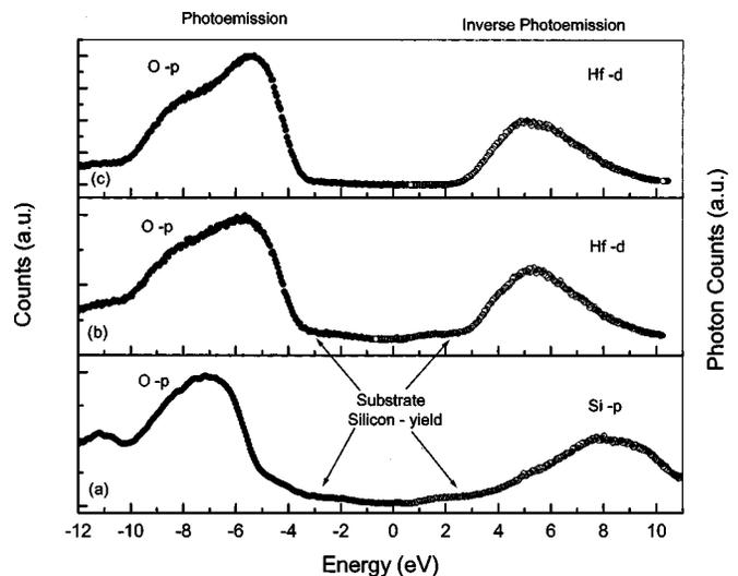
FIG. 6. Combined PES and IPES spectra of (a) 11 Å  $\text{SiO}_x\text{N}_y/p\text{-Si}$ , (b) 10 Å  $\text{HfO}_2/\text{SiO}_x\text{N}_y/p\text{-Si}$ , and (c) 28 Å  $\text{HfO}_2/\text{SiO}_x\text{N}_y/p\text{-Si}$ .
