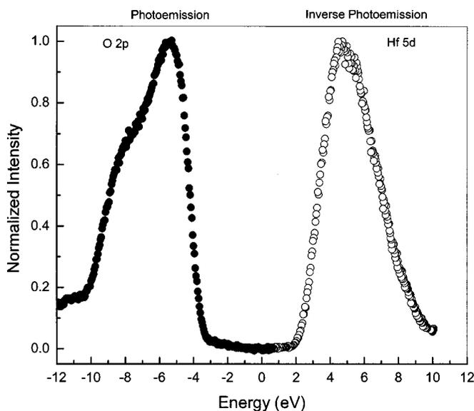
FIG. 2. Combined photoemission (●) and inverse photoemission (○); spectra of a 28 Å HfO<sub>2</sub>/SiO<sub>x</sub>N<sub>y</sub>/p-Si gate stack.
