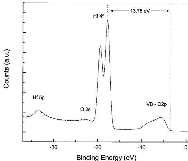
FIG. 1. Soft x-ray photoemission spectra of valence band region for a 28 Å HfO<sub>2</sub>/SiO<sub>x</sub>N<sub>y</sub>/p-Si gate stack.
