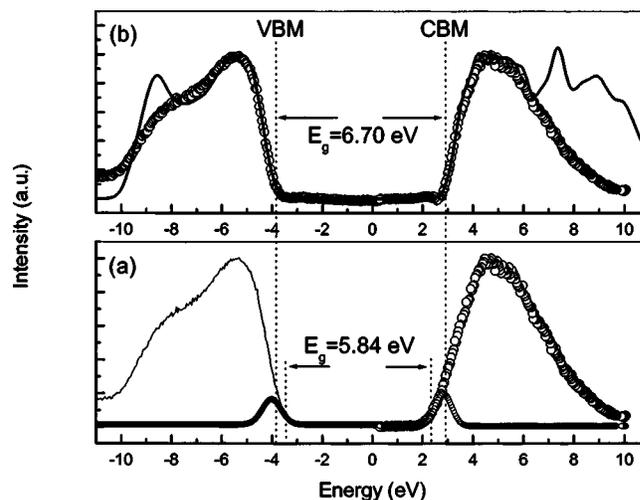
FIG. 8. (a) Densities of states of monoclinic  $\text{HfO}_2$  as determined by PES and IPES, the Gaussian peaks roughly model the presence of occupied and unoccupied band-tail/defect states in the vicinity of the VBM and CBM. (b) The fit between theoretical and experimental DOS improves after the band tail states subtracted from the measured DOS.
