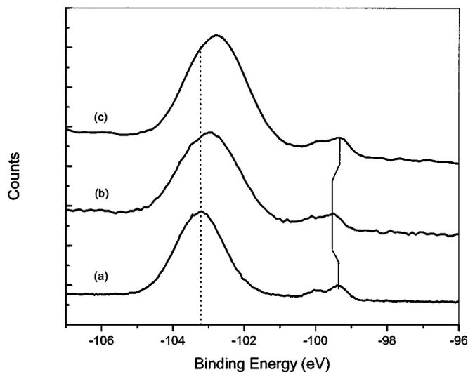
FIG. 7. SXPS spectra of Si  $2p$  region of (a)  $\text{SiO}_x\text{N}_y/p\text{-Si}$ , (b) as-deposited  $\text{HfO}_2/\text{SiO}_x\text{N}_y/p\text{-Si}$ , and (c)  $\text{HfO}_2/\text{SiO}_x\text{N}_y/p\text{-Si}$  after FGA.
