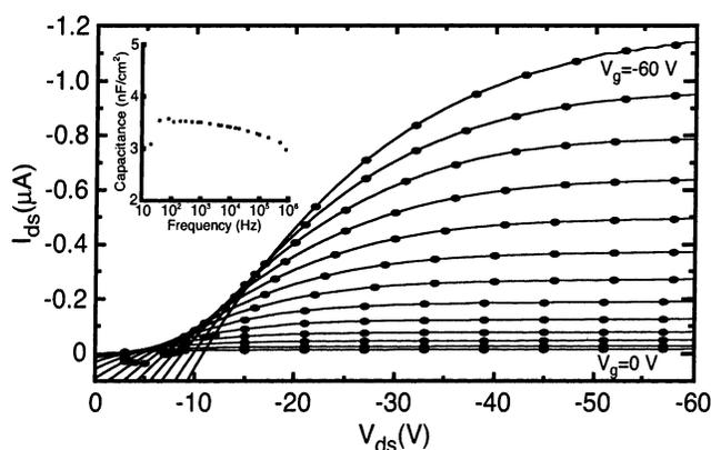
**Figure 2.** Current–voltage characteristics of an FET produced by direct deposition of the semiconductor layer and Au drain/source electrodes over an SI-ROMP polynorbornene dielectric layer grown from a Au gate electrode. The drain bias was swept from 0 to  $-60$  V at gate biases between 0 and  $-60$  V in  $-5$  V steps. Inset shows capacitance of a polynorbornene capacitor as a function of frequency. The leakage current is due to the unpatterned gate and organic semiconducting layers.
