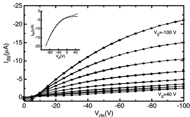
**Figure 1.** Current–voltage characteristics of an FET produced by lamination, containing an SI-ROMP polynorbornene dielectric layer. The drain bias was swept from 0 to  $-100$  V and back at gate biases between 40 and  $-100$  V in  $-20$  V steps. Inset shows drain current as gate voltage was swept from 40 to  $-100$  V and back.
