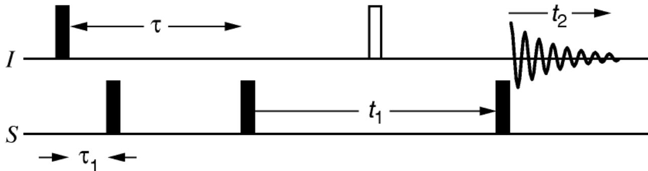
*The delay  $\tau_1$  is set to  $1/2(^1J_{IS})$  and  $t$  is the usual long delay corresponding to long range coupling. The one bond coupling generate its own antiphase coherence that is converted into MQC by the first 90o pulse on the S-spin. The experiment is done twice once with this pulse along (x)-axis and again along (-x)-axis and added to suppress the direct peak.*
