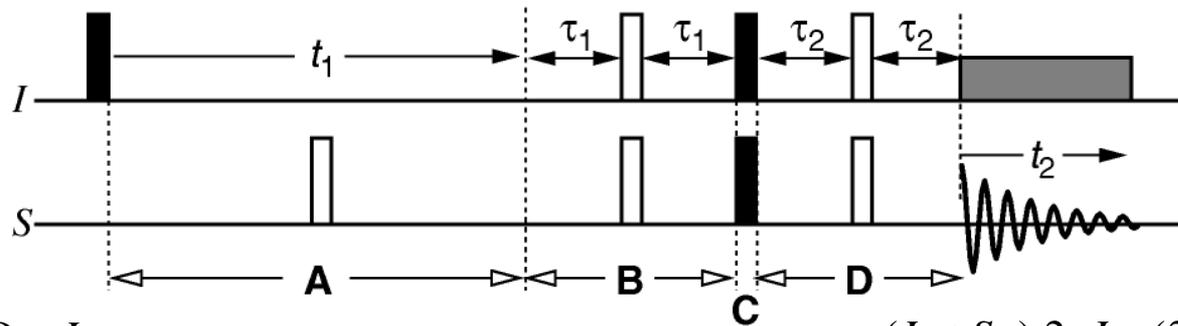
$$I_z \xrightarrow{\frac{\pi}{2}I_x} -I_{1y} \xrightarrow{\Omega_I t_1 I_{1z}} -I_y \cos(\Omega_I t_1) + I_x \sin(\Omega_I t_1) \xrightarrow{\pi(I_x + S_x), 2\pi J_{IS}(2\tau_1)I_z S_z} \rightarrow$$
