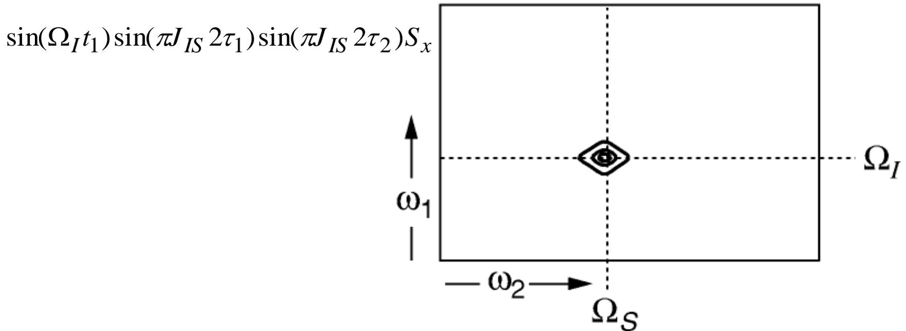
*A peak at  $\Omega_I$  in  $\omega_1$  and  $\Omega_S$  in  $\omega_2$  appear. It is the cross peak equivalent of the COSY spectrum. There is no diagonal peak as we are correlating two different nuclei.*
